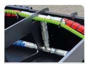
Hydraulic run down protection - anti-cavitation valve
