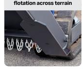
Serrated round blade carrier with increased mass and balance for smoother cut
