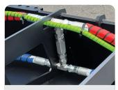
Hydraulic run down protection - anti-cavitation valve
