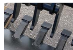
High tensile tynes with 10 mm Bisalloy wear tips
