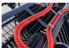
Protective rear spill guard with high visibility mesh
