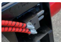
High torque hydraulic motor and pressure relief valve
